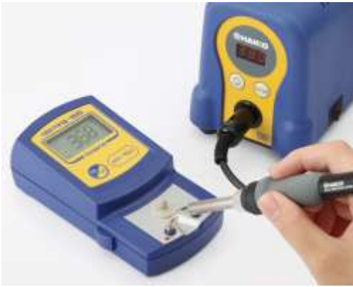
Measuring tip temperature with a tip thermometer (HAKKO FG-100)
