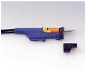
(1) Detach the nozzle remover
